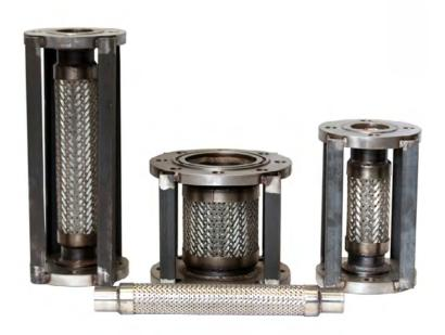
Flexible hoses are designed to absorb vibration and noise, compensate for thermal expansion and contraction and to relieve piping stress due to minor outlet misalignments. They are easy to install and eliminate the need for many fittings and extreme accuracy when roughing in. Flexible hoses are available in standard sizes: ¼" – 30".
